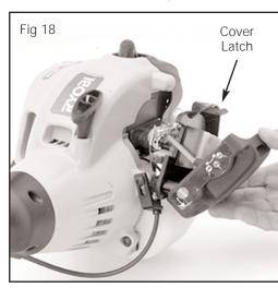
Remove and wash the filter with soap and water. Allow to completely air dry before replacing the filter. After replacing the filter secure the air filter cover.
